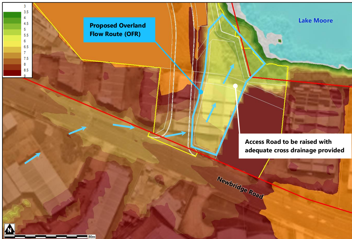
Plate 4.1 Topography along the Proposed Overland Flow Route Relative to the 'sag' along Newbridge Road
